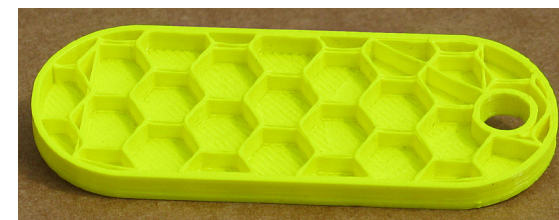
Countersunk hole & thread test print. Drill & die both required post printing.
