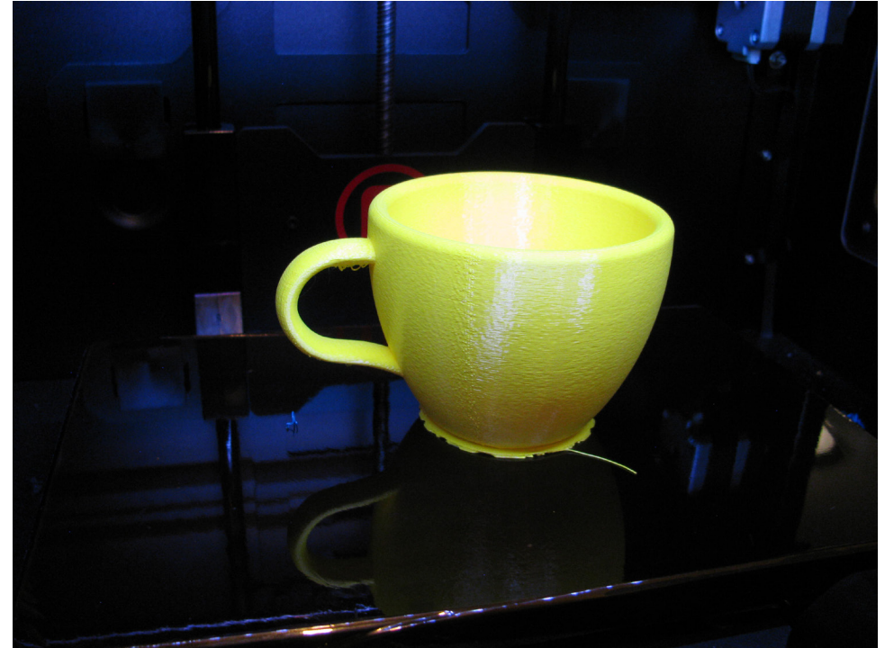
Very little hangers, just a bit off the upper inside of the finger hole due to lack of supports.
