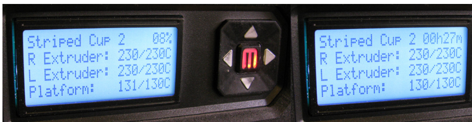
Rafts laid down for cup and supports. Base of cup appears. 8% at 27 Minutes
