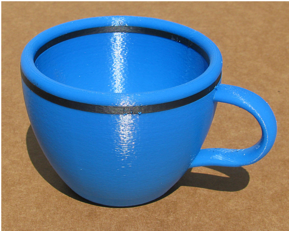
Dual color printing using MakerBot Replicator 2X
